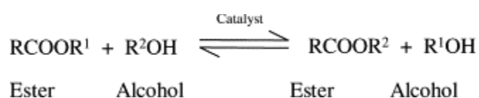
Figure 2. General equation of catalysed transesterification (Meher et al., 2006).
