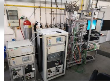
Measurement of burners and exhaust gas investigations (MS, GC, FTIR, FID, gas analyzer)
