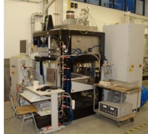
600°C combined 2.45 GHz and 5.8 GHz microwave/ hot air heated furnace with large chamber
