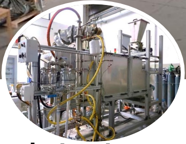
Intermediate/Slow Pyrolysis - Spyro 2-3 kg/h
